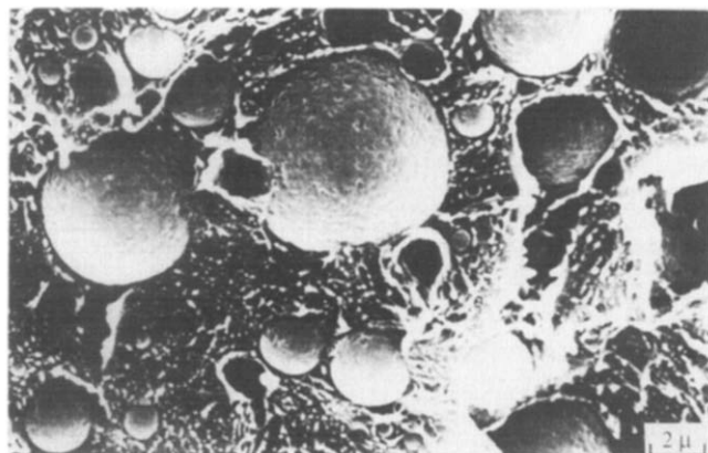
Figure 5 Secondary electron image of a cryogenically fractured PPSH/PE blend ( \phi_{PE}=0.53 ), showing the orange-peel appearance of PPS particle surface
